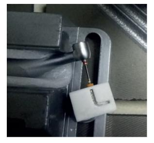
**Figure 1** Device created for the cyclic fatigue resistance tests of the rotary instruments.
