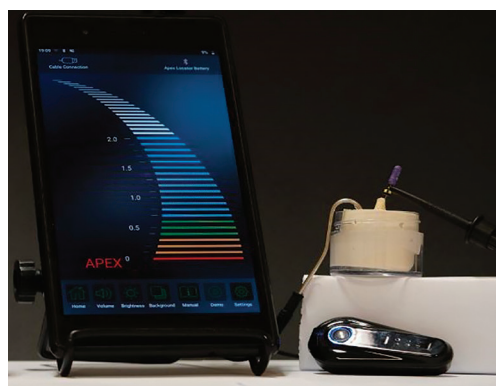
Figure 4 The display unit connected via Bluetooth to Wirele-X device with the screen showing the red bar at the mark “0”.
