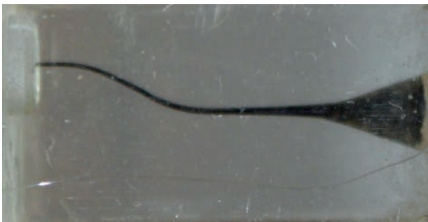
Figure 1 Photo of resin block before instrumentation where injected with black ink to improve the color contrast.
