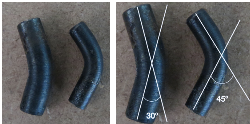
Figure 1 Stainless steel devices fabricated in an angled tube format and used to simulate a root canal.
