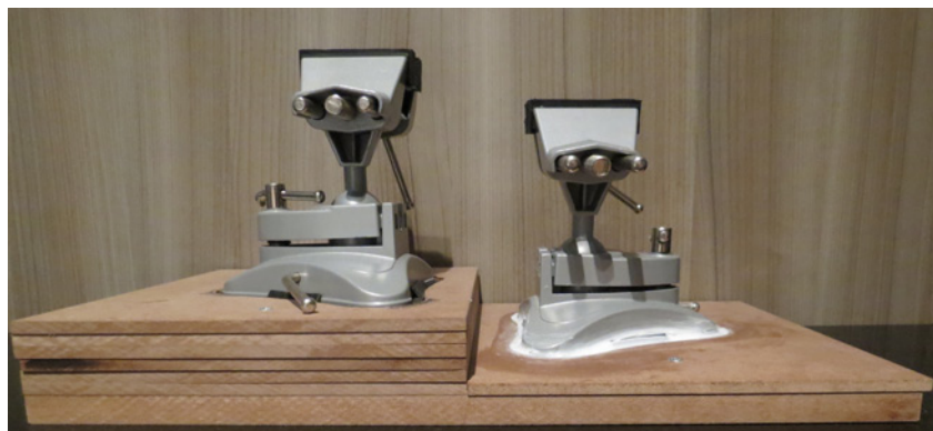
Figure 2 Support created with the two mini-vises for the experiment.
