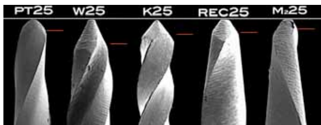
Figure 19 Different distances between the tip of the instrument and the working diameter.
