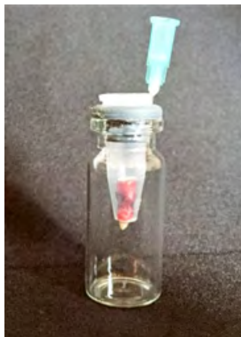
Figure 1 Bacterial leakage device composed of two chambers connected by the endodontically treated tooth.
