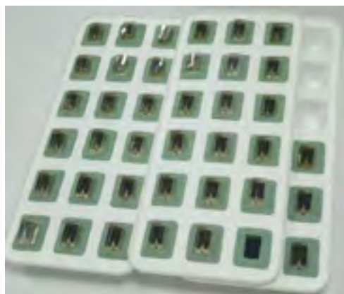
Figure 1 Preparation of the blocks in holders made with putty and ice cube tray.
