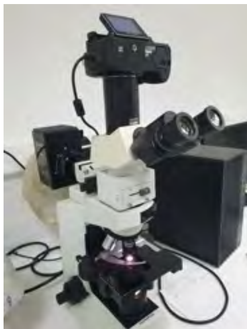
Figure 2 Olympus optical microscope at 1.25x/0.04/FN 26.5 magnification.
