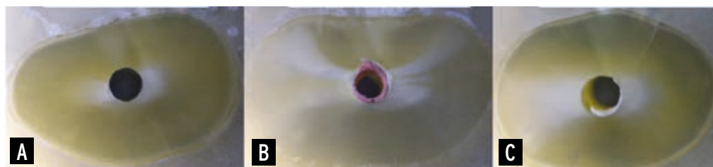
Figure 1 Visualization of failure types after POBS testing under a stereo microscope A) Adhesive failure, B) Cohesive failure, C) mixed failure.
