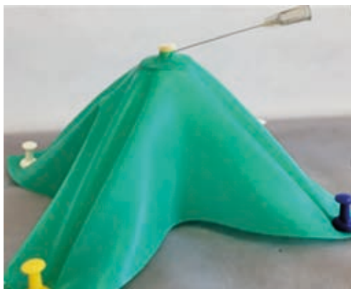
Figure 2 A modification of the experimental setup developed by Meyers and Montgomery was used for debris collection.
