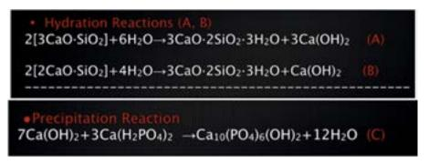
Figure 1 Hydration reaction of bioceramic material in contact with water (A and B). Precipitation reaction of the bioceramic (C).
