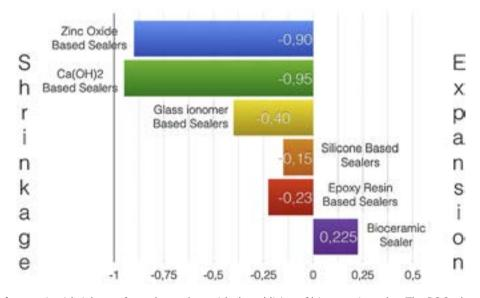
**Figure 7** Table of expansion/shrinkage of popular sealers with the addition of bioceramic sealer. The BC Sealer expands slightly on setting but does not shrink.
